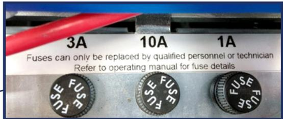
The fuses can only be replaced by qualified personnel or technician, refer to below fuse specifications for replacement guide.
