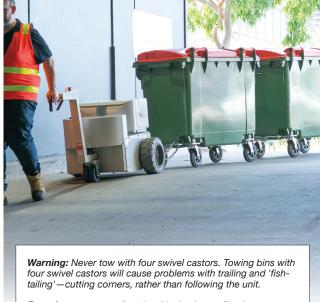
For safety purposes, directional lock tabs are fitted to your bin's existing rear swivel castors to enable controlled steering and towing in a straight line.
